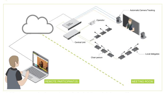
Typical Plixus Gateway setup where the gateway is connected to the Cloud, the Central Unit, the screen and the cameras
